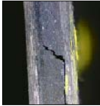
Figure 2: Interfacial crack extending from the tip of a transverse microcrack.
