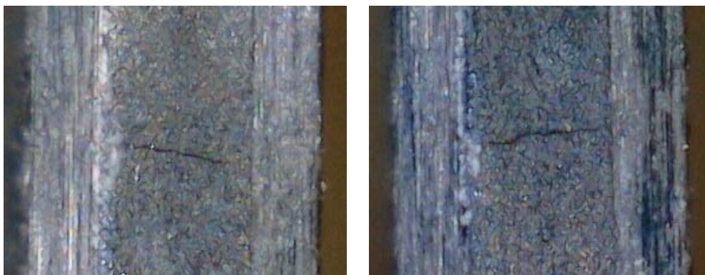
Figure 1: Examples of microcracks in transverse (90°) plies of a cross ply [0/90] s laminate.
